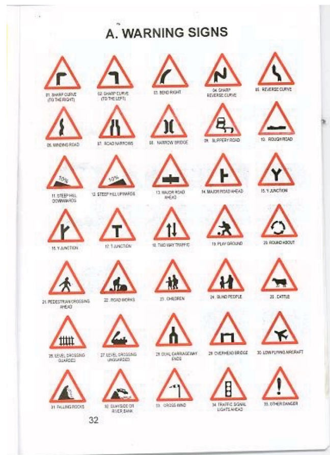
Figure 3: Warning signs in the Ghana Highway Code
