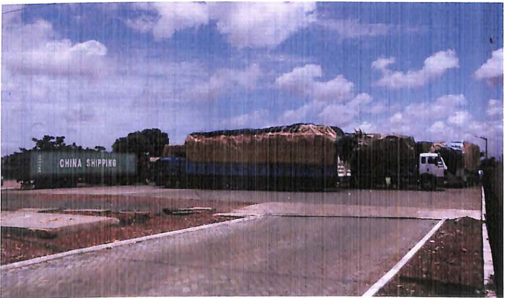
Figure 5: Overloaded trucks parked at the Tema Motorway axle load control station. Source, Appiah, 2015
