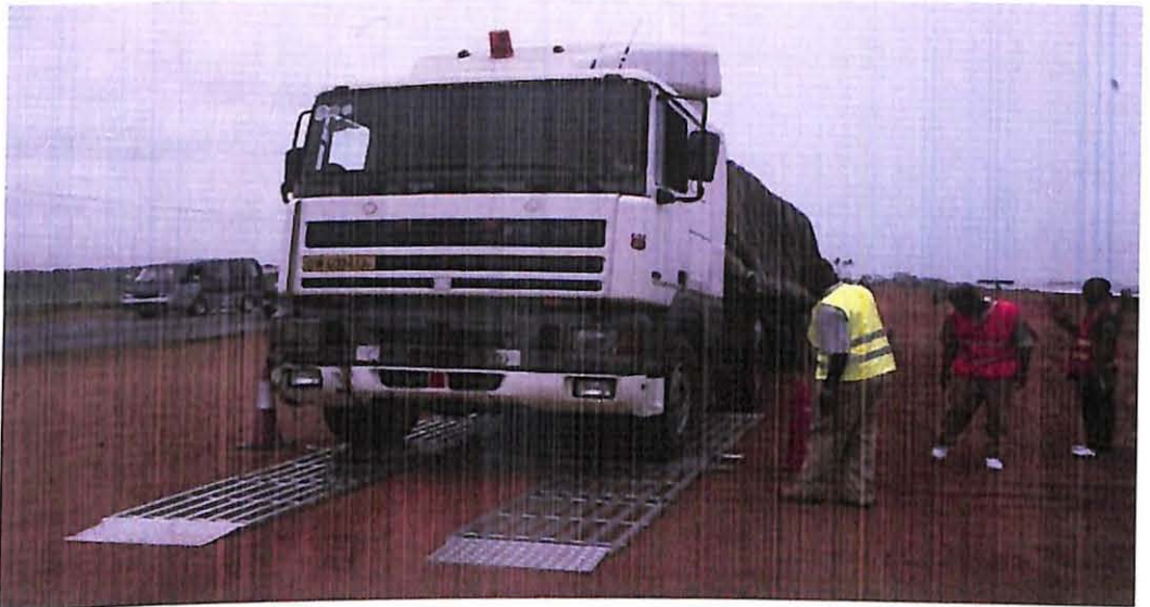
Figure 10: A truck loaded with cement going through a mobile weighbridge
