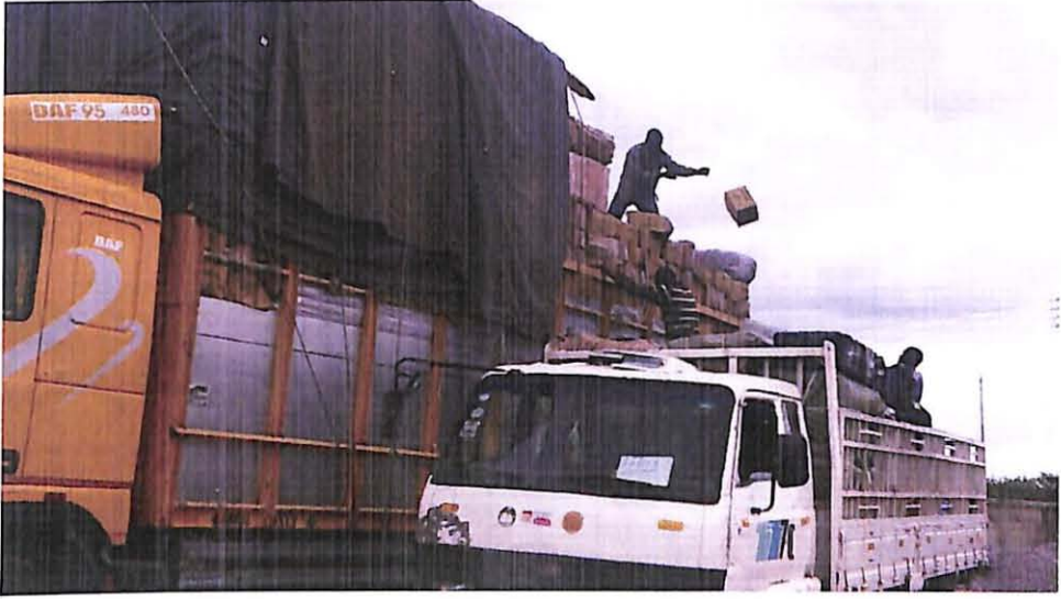
Figure 7: Load being shed-off from an overloaded truck to an empty vehicle. Source, GHA
